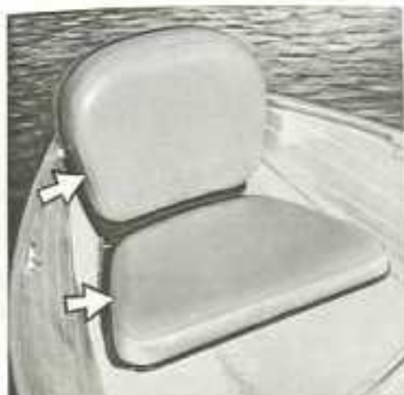
BOAT SEAT: This project was made of vinyl material, with vinyl welts. 4" of foam rubber was used for padding. Seat fits bow of boat.
